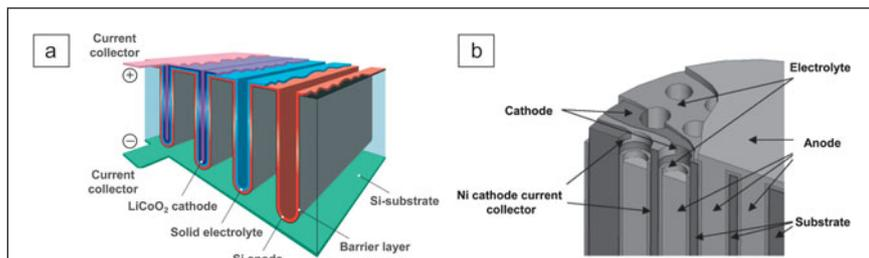
**Figure 2.** Schematic of 3D battery architectures that amplify the area of thin-film batteries: (a) use of a silicon trench substrate coated with a barrier layer to prevent any reactions of the substrate with Li-ions (Reprinted with permission from Reference 12. ©2007, Wiley-VCH Verlag GmbH & Co.); (b) use of a perforated substrate of glass or silicon (Reprinted with permission from Reference 11. ©2005, IEEE).
