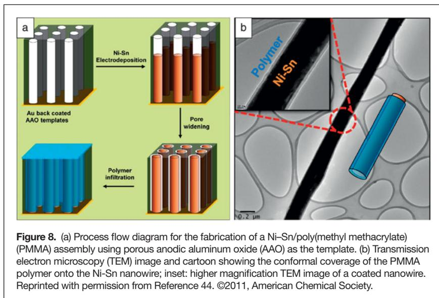
**Figure 8.** (a) Process flow diagram for the fabrication of a Ni-Sn/poly(methyl methacrylate) (PMMA) assembly using porous anodic aluminum oxide (AAO) as the template. (b) Transmission electron microscopy (TEM) image and cartoon showing the conformal coverage of the PMMA polymer onto the Ni-Sn nanowire; inset: higher magnification TEM image of a coated nanowire. Reprinted with permission from Reference 44. ©2011, American Chemical Society.
