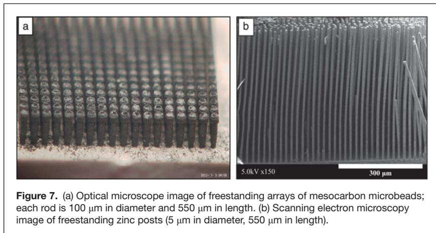
**Figure 7.** (a) Optical microscope image of freestanding arrays of mesocarbon microbeads; each rod is 100  $\mu\text{m}$  in diameter and 550  $\mu\text{m}$  in length. (b) Scanning electron microscopy image of freestanding zinc posts (5  $\mu\text{m}$  in diameter, 550  $\mu\text{m}$  in length).
